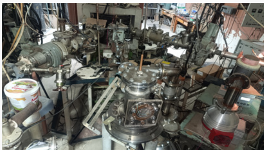
Fig. 2. Universal camera docked to the central terminal of the EG-2 accelerator
